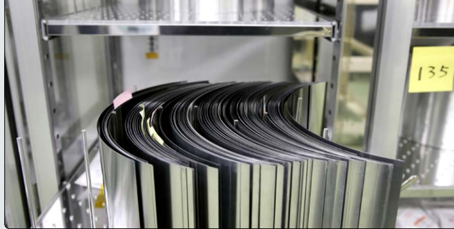
硬X線望遠鏡。多層膜で高エネルギーX線を集光結像する。 「ひとみ」衛星にも搭載。性能向上型や検出器も開発中。 A hard X-ray telescope, which is a grazing incident angle optical device, that focuses hard X-rays. A higher resolution version is under development.
