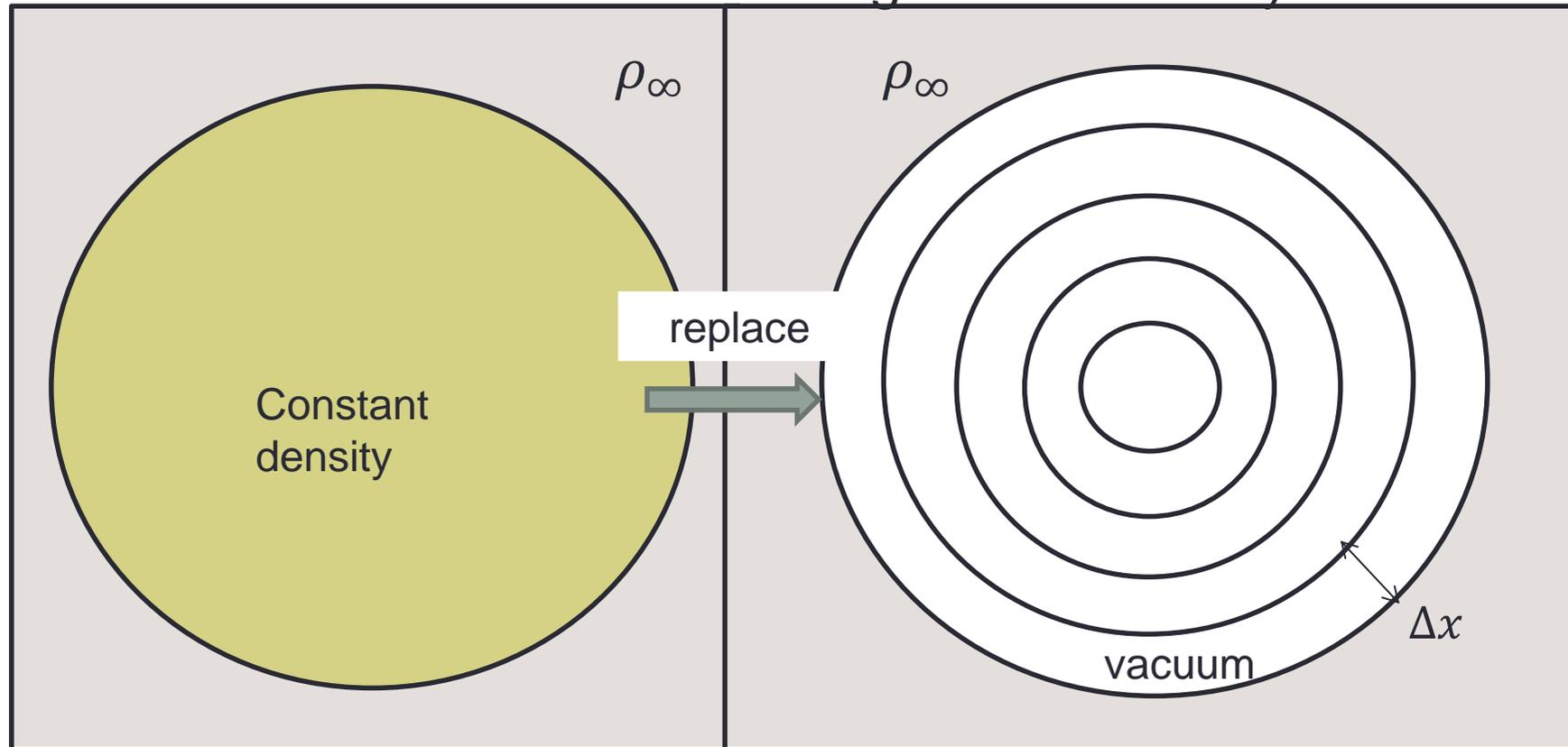
Each shell is infinitely thin, has same density and separated by vacuum regions with equal intervals.
