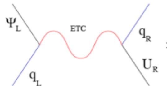
Feynman diagram illustrating an Extended Technicolor (ETC) interaction. A fermion line labeled  $\Psi_L$  and  $q_L$  enters from the left, and a quark line labeled  $q_R$  and  $U_R$  exits to the right. Between them is a red wavy line representing an ETC interaction. The resulting expression is  $\frac{g_{ETC}^2}{M_{ETC}^2} (\bar{\Psi}_L U_R)(\bar{q}_R q_L)$ .
