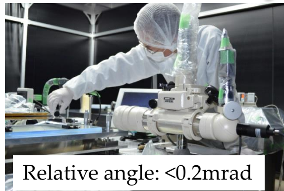
(1) Alignment (using the laser displacement sensor, autocollimator)
