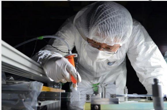
(2) Put glue on the surfaces & UV Light Curing
