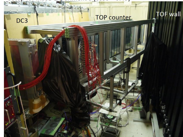
Setup for IRS3B Experiment 3 ( \cos\theta = 0.43 )
