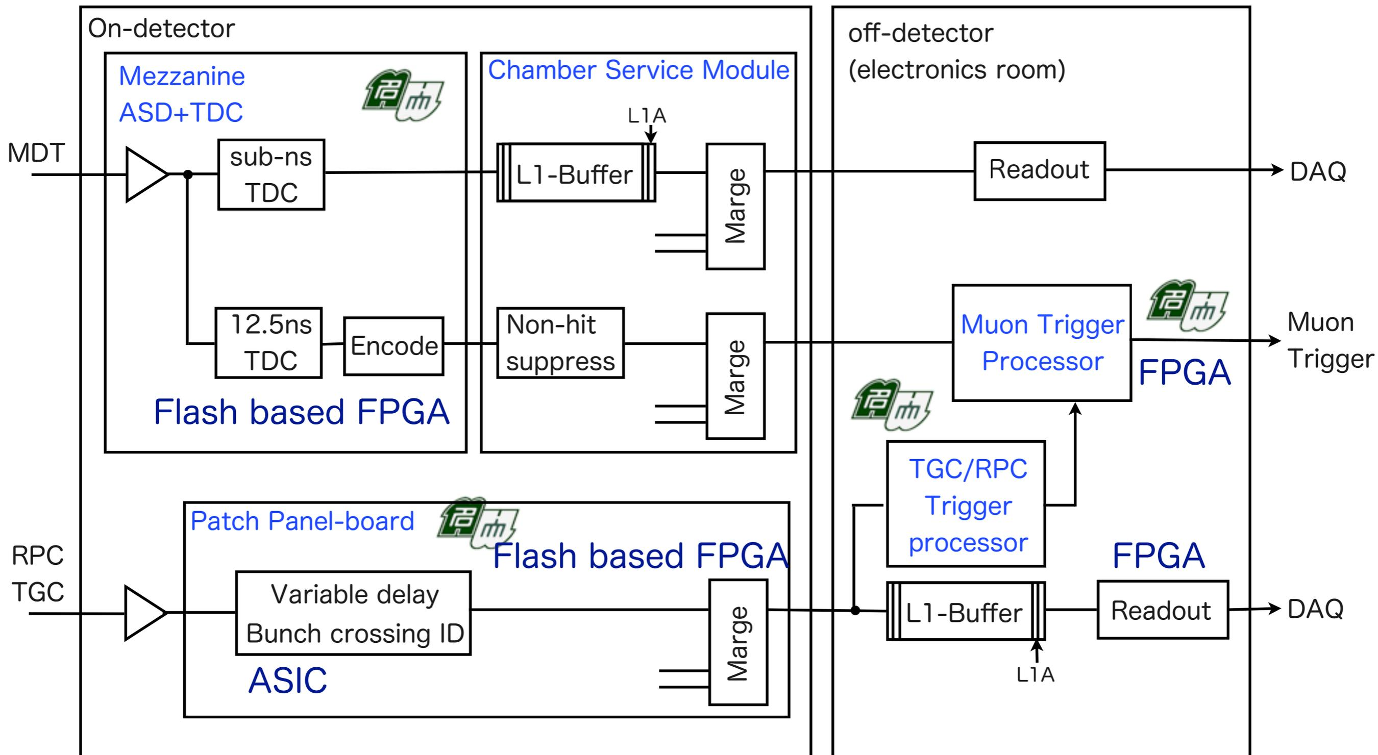
Most of electronics are developed by FPGA.
