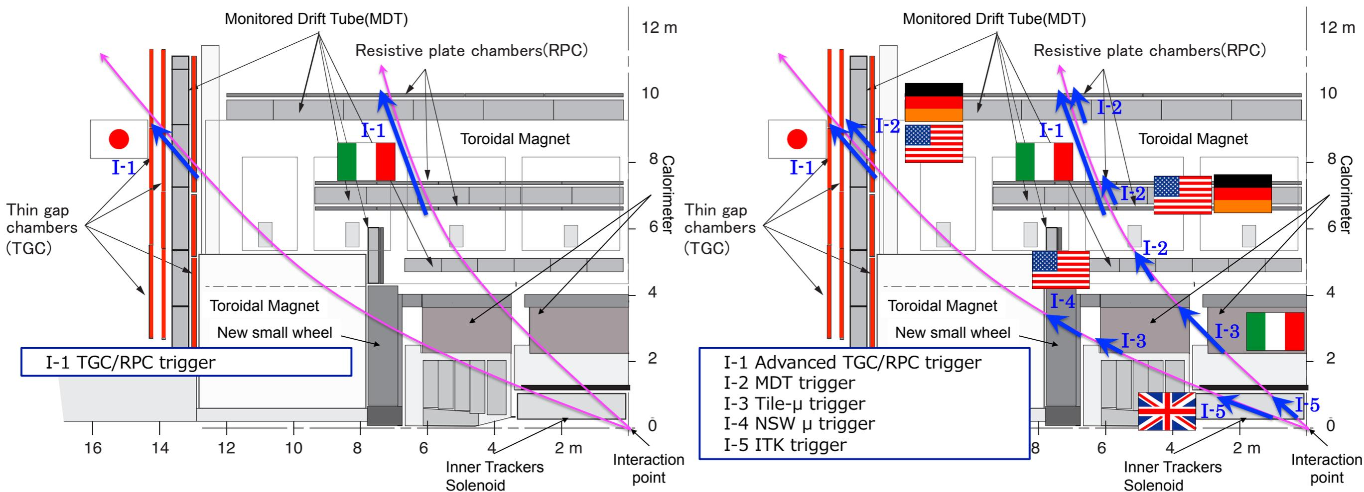
Muon trigger upgrade for HL-LHC consists of
