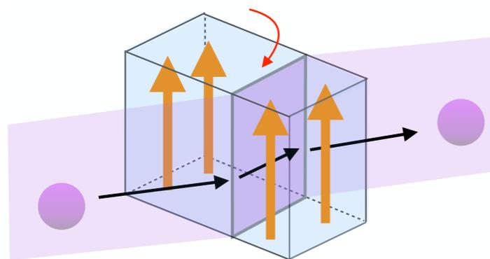
Pendellösung interference fringes with pulsed neutrons was observed clearly to be basis of crystal-EDM technique.
