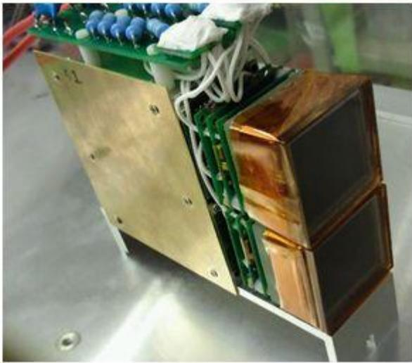
16 outputs of each PMT were merged into 4 at the PMT socket to reduce the number of channels (little impact on the PID performance)
