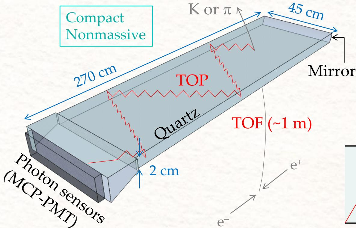
Cherenkov photons generated in the quartz bar travel in the bar as they are totally reflected on the quartz/air boundaries.
