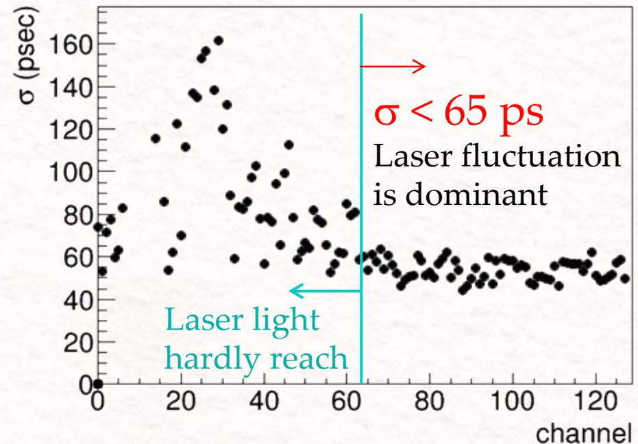
The timing resolution of the system was proved to be good.
